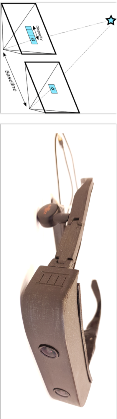
Figure 1, baseline is the distance between the camera lenses.
