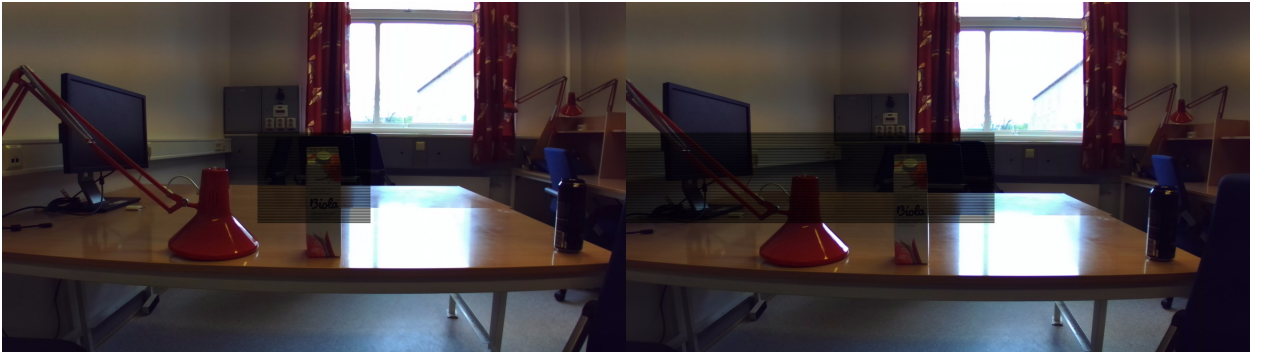
Figure 5.1.7: Stereo camera frame captured from the ZED Mini. The marked area is a set of 160 horizontal lines with a vertical spacing of 1px. The total height covers 320px.
