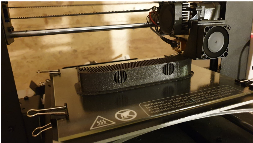
Figure 5.5.3: The prototype stereo camera housing in the midst of being printed with black PLA from Prusa Research .
