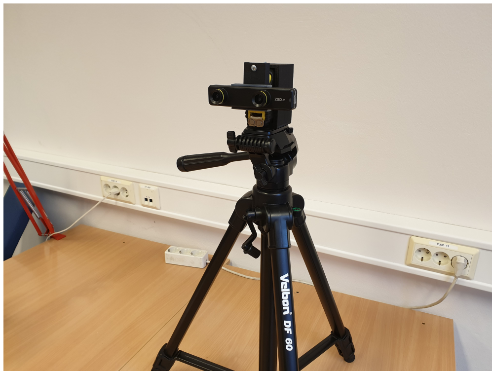
Figure A.6: Tripod with the custom 3D printed holder, and the ZED Mini camera attached.
