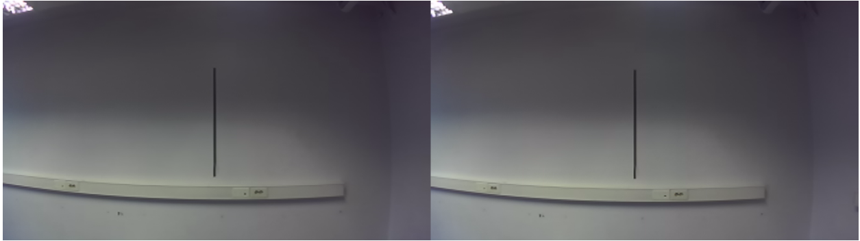
Figure 5.2.1: One of the calibration images, taken at 200cm from a white wall with black tape as the target-object. The frame is captured with resolution 1344x376.
