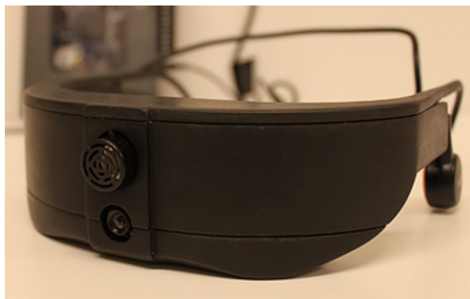
Figure 1.2.1: The current Colorophone design as of January 2019, consisting of a 3D printed housing which contains an ultrasonic sensor, an RGB camera, and a set of bone conductive headphones. 1
