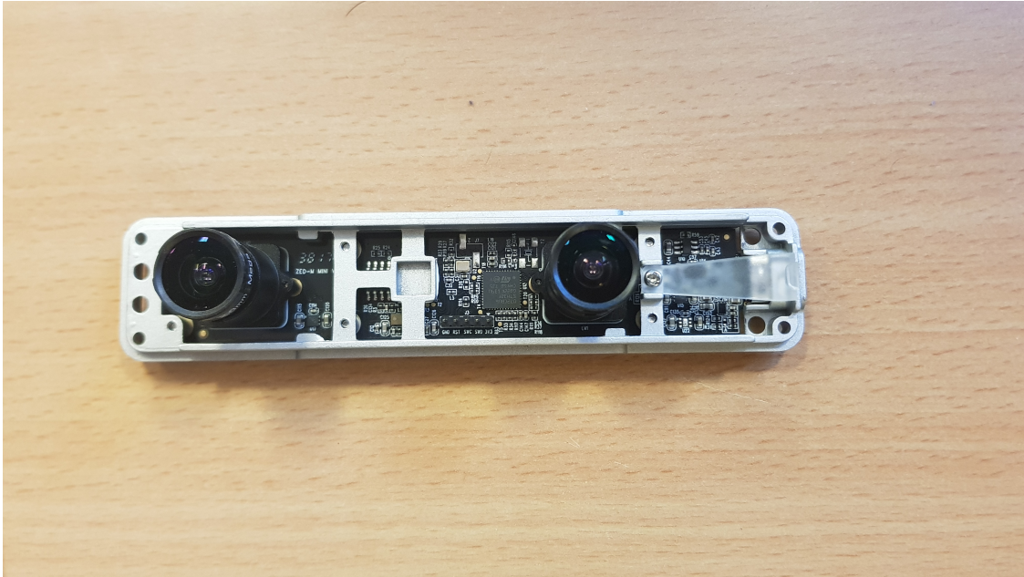
Figure 5.4.3: The ZED Mini internals.
