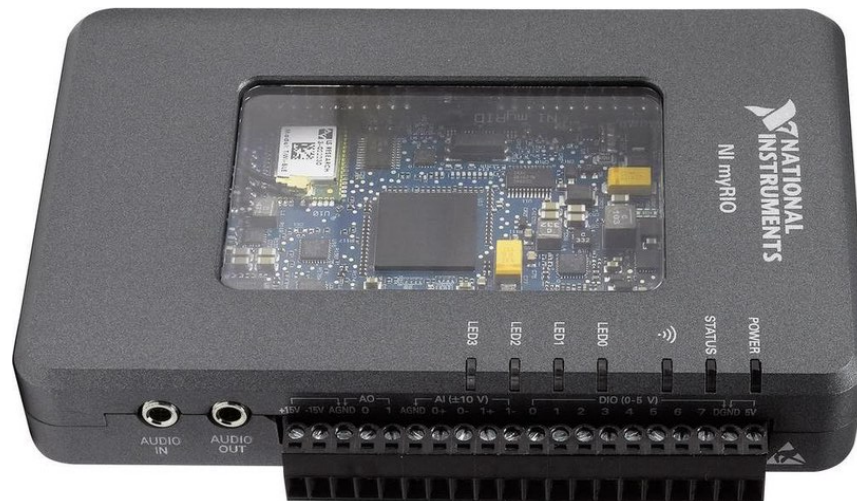
Figure A.4: The myRIO device by National Instruments. 6
