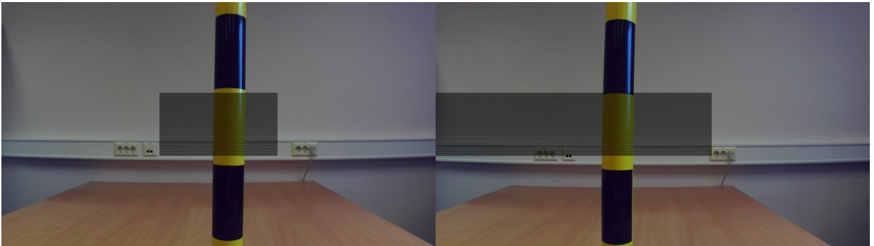
Figure 5.1.3: Stereo camera frame captured from the ZED Mini. The actual, real distance to the object is 40cm. The marked area indicates the distance calculation area, where the input data for distance calculation is extracted.
